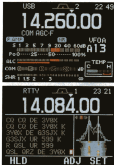
CLOCKWISE FROM LEFT: PHOTO 6: IC-7000 BAND SCOPE DISPLAY PHOTO 7: THE MULTI-FUNCTION METER DISPLAY PHOTO 8: IC-7000 RTTY DECODER DISPLAY PHOTO 9: IC-7000 SWR PLOT DISPLAY
