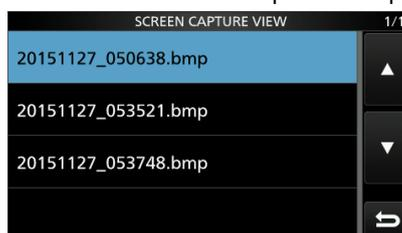
Ⓜ While a screen capture is displayed, you can scroll through all the screen captures by rotating **(MULTI)**.
