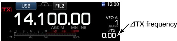
2. Set the ΔTX frequency to match the receiving station's frequency.
