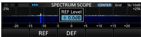
4. Rotate (**MAIN DIAL**) to adjust the level.
