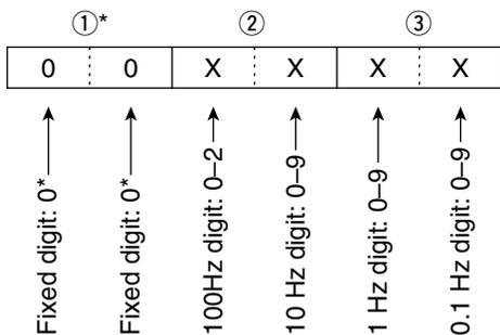
\*Not necessary when setting a frequency.
