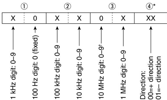
\*1 There is no need to enter the transverter offset frequency setting.
