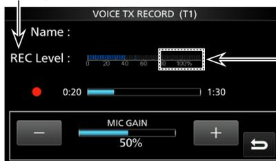
Adjust the Mic gain so that the “REC Level” meter does not reach 100%
