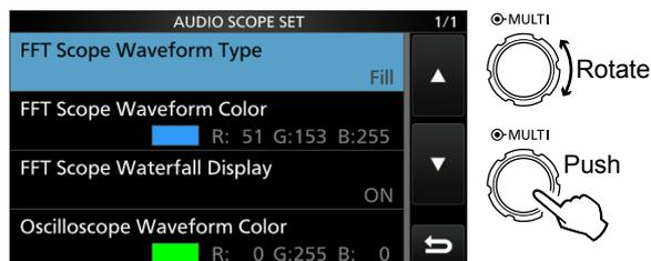
4. Rotate **(MULTI)** to select the option or set the level, and then push **(MULTI)**.
