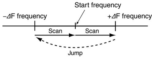
Repeatedly scans within the ΔF span area. The scan starts from the center frequency.
