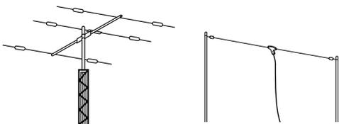
Connect a 50 Ω antenna for the HF, 50/70 MHz frequency bands.
