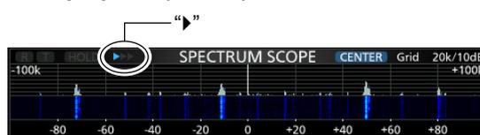
4. To exit the SPECTRUM SCOPE screen, push (**EXIT**).
