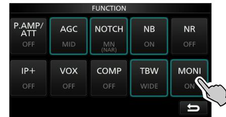
5. Adjust MONITOR to the clearest audio output between 0% and 100%, while speaking at your normal voice level.
