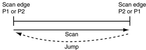
Repeatedly scans between two Scan Edge frequencies. The edge frequencies are preset in P1 and P2 as the default.
