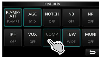
11. While speaking into the microphone at your normal voice level, adjust the Speech Compressor level to where the COMP meter reads within the COMP zone (10 to 20 dB range).
