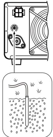
**⚠ WARNING! NEVER** connect the [GND] terminal to a gas or electric pipe, since the connection could cause an explosion or electric shock.
