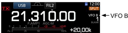
The offset between transmit and receive while holding down **[XFC]**.
