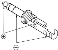
When connecting a CW paddle and using the internal electronic keyer.
