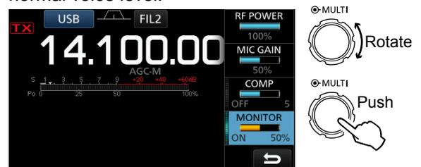
**NOTE:** When using the VOICE DELAY (p. 4-10), turn OFF the Monitor function. Otherwise the transmitted audio will echo.
