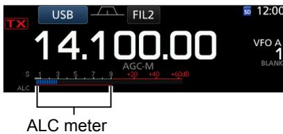
6. Adjust the MIC GAIN (p. 3-11) to where the ALC meter reads within the 30 to 50% range of the ALC zone.
