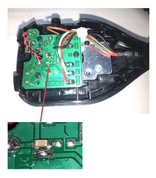
3 ---- With the help of a soldering iron remove the resistor, and shorting two pads with a drop of tin.
