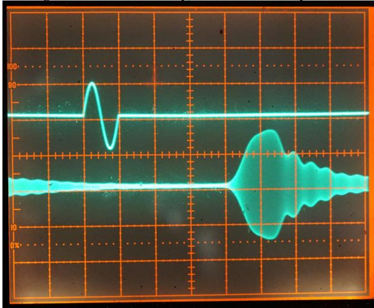
Figure 36: Transmit latency, MID TBW. Latency 4.2 ms.
