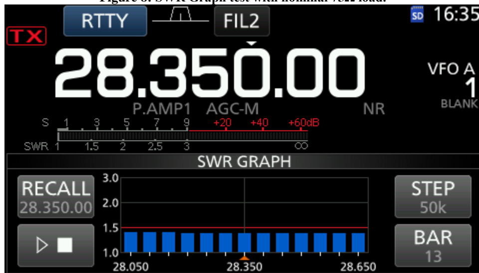
Figure 8: SWR Graph test with nominal 75Ω load.
