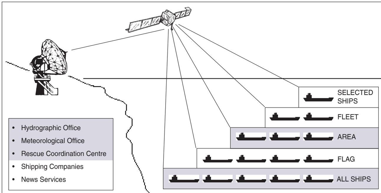
Figure 13 — Basic concept of the Inmarsat Enhanced Group Call system (the shaded area indicates functions of the SafetyNET service)
