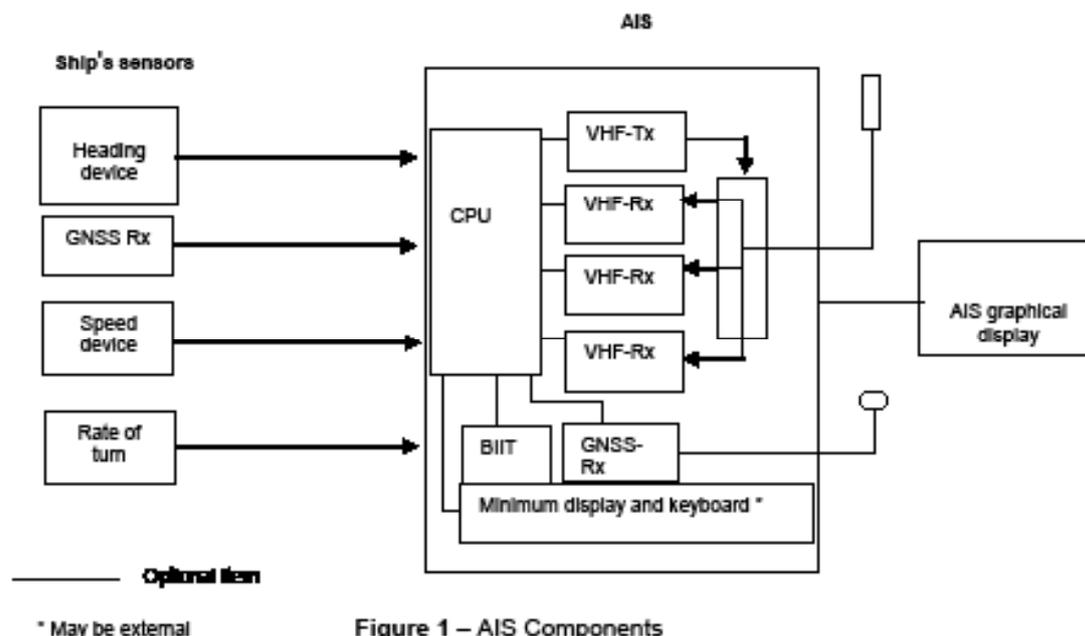
Figure 1 – AIS Components
