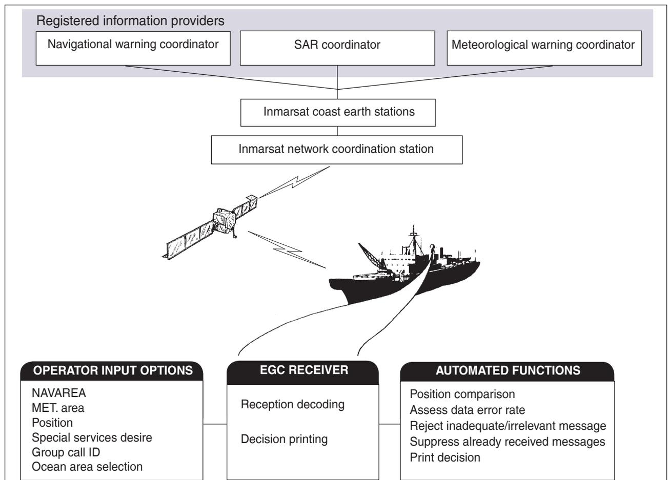
Figure 15 - International SafetyNET Service System Concept
