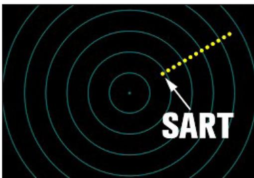
Figure 24 — SART Radar Display
