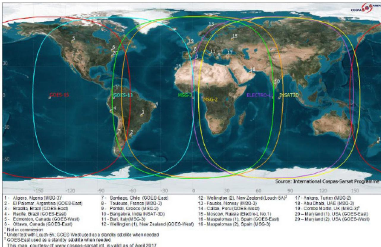
Figure 21 — 406 MHz GEOSAR Satellite Coverage and GEOLUTs
